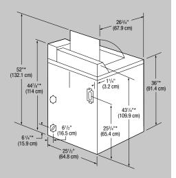
\* Dimensions will vary according to adjustment of leveling legs; add ½" (1.3 cm) minimum.
