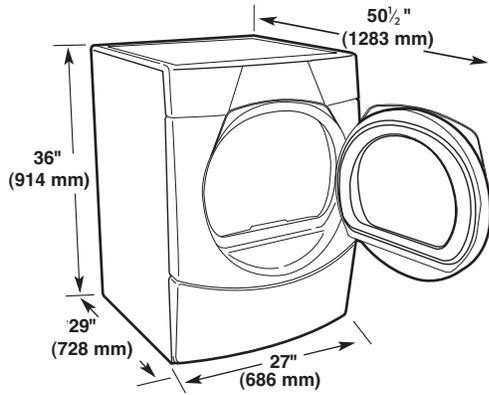
**NOTE:** Most installations require a minimum 5" (127 mm) clearance behind the dryer for the exhaust vent with elbow. See "Venting Requirements."
