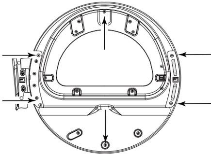
4. Lift the inner door assembly off the outer door assembly.
