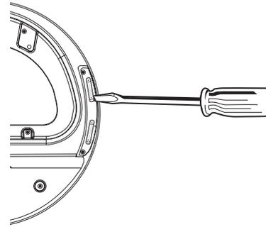
2. Remove the 4 screws that attach to the inner door hinge and move the hinge to the other side. Reinstall the 4 screws.
