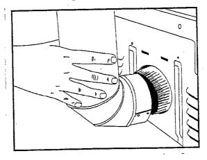
Tip for tight installations: install a section of exhaust system to the dryer before moving the dryer in place. Use duct tape to secure this section to the dryer but do not cover louvers in dryer cabinet.
