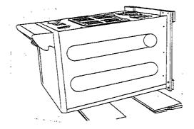
2. Remove the crate wires holding the crate base to the base frame. This can be done with a screwdriver.
