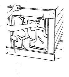
3. Loosen the leveling locking nuts and install the vinyl feet.
