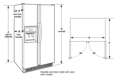
Dimensions "C" and "D" include rollers extended ¾" (1.9 cm).
