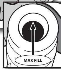
Dilute liquid fabric softener by filling the dispenser with warm water until liquid reaches the underside of the rim. See "Max Fill" line arrows.
