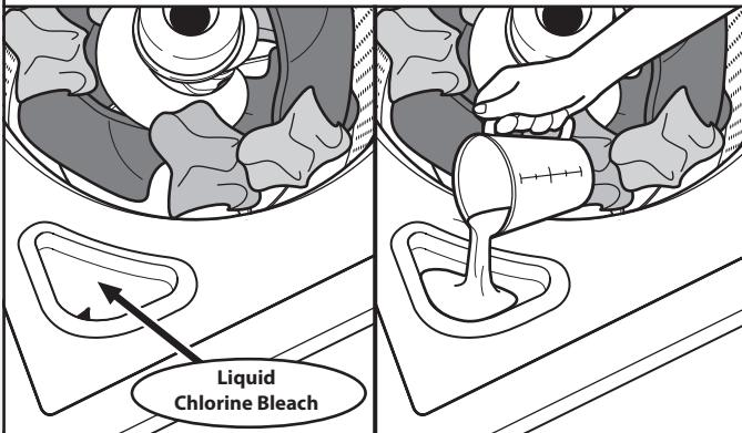
Do not overfill, dilute, or use more than 1 cup (236 mL) of liquid chlorine bleach.
