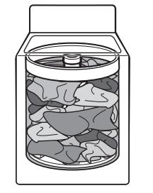
**IMPORTANT:** Do not tightly pack or force items into washer. Items need to move freely for best cleaning and to reduce wrinkling and tangling.
