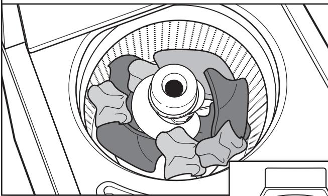
Load garments in loose heaps evenly around basket wall. For best results, do not pack the load tightly. Do not wrap large items such as sheets around the agitator. Load them in loose piles around the sides of the basket. Try mixing different-sized items to reduce tangling.
