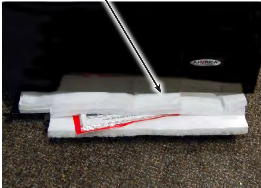
Figure 8 - Tech Sheet located behind toe panel inside insulation folds.
